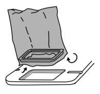
1 Push up on the underside of the bag support insert to remove. Then attach plastic bag as illustrated above.
