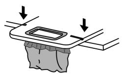
(3) Match marks on the platform with the table edge. Then push the plastic bag through to the underside as illustrated.
