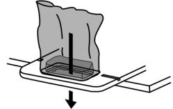
2 Place bag support insert into opening with about 1 to 2 inches of plastic bag turned up inside.
